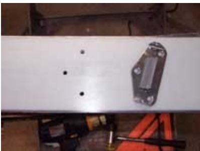
The touring bracket holes before counter sinking.
